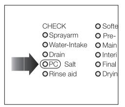
When the salt reservoir is empty, the "Salt" indicator lamp will light, notifying you that the reservoir should be refilled with reactivation salt.
